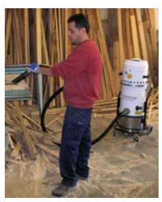
Wood manufacture, recovery from a belt saw.
